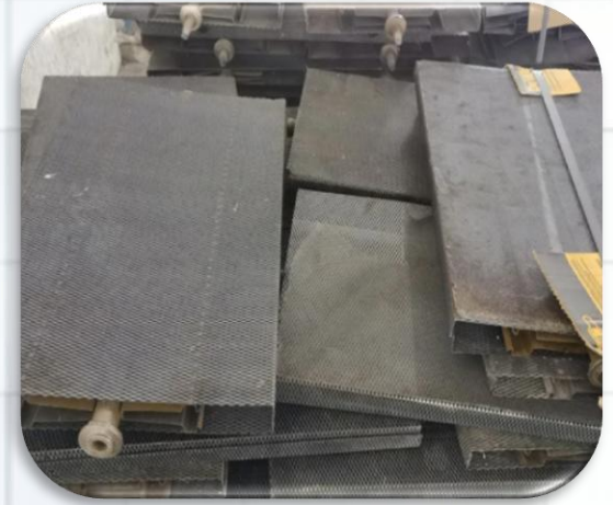
Titanium Mesh for PEM Electrolyzers
