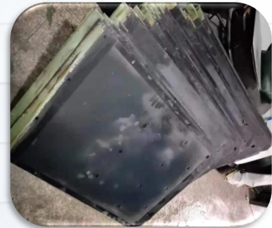
Nickel ruthenium mesh for PEM Electrolyzers
